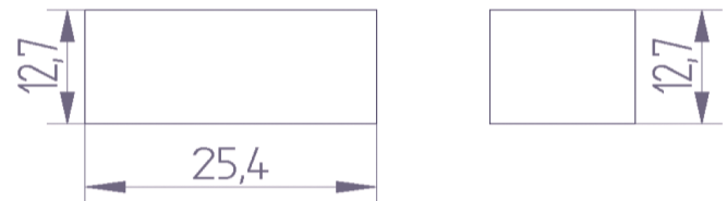
Fig. 5.2 Compression test specimen specification
